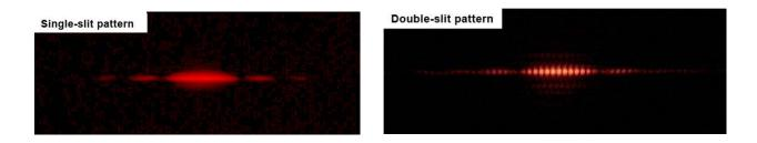
As the number of equally separated slits are increased, the center (interference maxima) becomes much brighter relative to the other bright spots. This is what diffraction grating simply manages to do: it increases the number of slits. However, in Raman Spectroscopy, this is not the reason why grating is used. There is another property of gratings which makes them useful. Consider the following figure where maxima (bright spots) are modeled for a diffraction grating:
