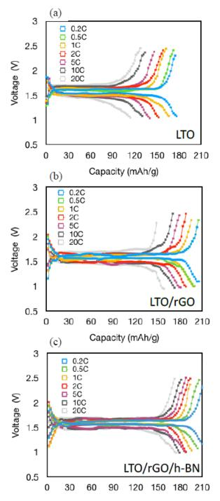
Figure on the left shows charge and discharge curves at different charging rates. (a) is for LTO, (b) is for LTO/r-GO composite, (c) is for LTO/r-GO/h-BN composite. Observe that adding r-GO to LTO improves capacity and adding h-BN to t-GO/LTO composite improves more. Especially at higher charging rates, h-BN makes the greatest impact. Therefore, composite with h-BN is superior. Different h-BN:GO Loading Conditions:
