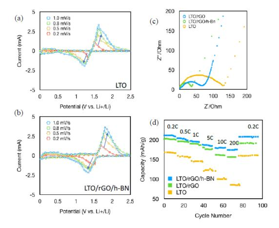
(a) is for LTO and (b) is for LTO/r-GO/h-BN composite. It is observed that (b) is the right-shifted version of (a) which means operates at higher voltage. Observe that (b) manages to reach higher current values and peaks are wider, meaning that there is a wider operating voltage range for LTO/r-GO/h-BN.
