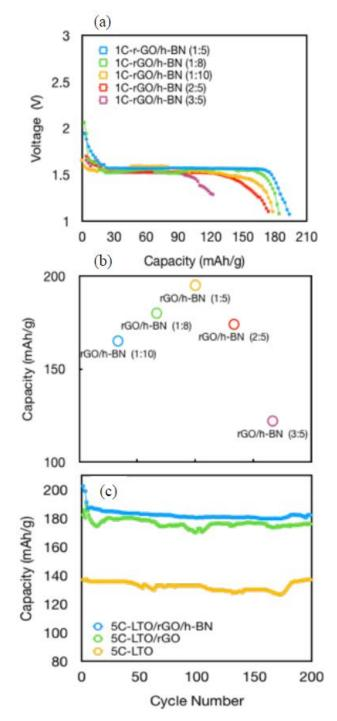
(a) is discharge curve for different h-BN loading conditions. Observe that the largest capacity is reached for the loading 1:5.
