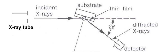
So, when constructive interference happens, diffracted rays amplify each other (instead of cancelling) and we get an X Ray at the same wavelength. This wave is then detected by the detector at a specific angle. Since we require a constructive interference, we also need to understand when a constructive interference happens. The answer to this question is the condition when Bragg's Law is satisfied. It is stated as follows:
