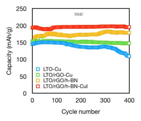
Lastly, to overcome lowered specific capacity degradation, Cu is added, which in result allows better electron transport and stability. As observed from the figure, h-BN composite (without Cu) is superior to all other composites except h-BN composite with Cu in terms of capacity. Therefore, it is concluded that h-BN addition here is also improving and addition of Cu improves the battery even more. Cu and h-BN can operate properly together.
