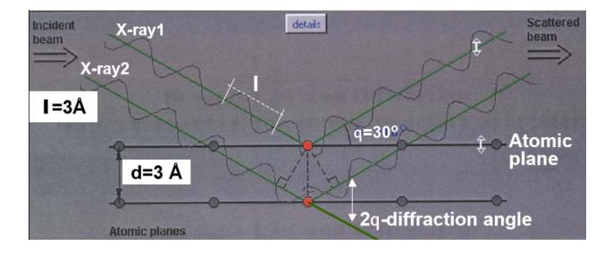
This interaction causes interference pattern because the length of the paths traced by both rays are different. This interference can be in two opposite manners: *destructive* and *constructive*. In XRD Spectroscopy, we are interested in the constructive interference. This is because we use a detector that detects the photons falls on it. Consider the following figure of XRD before we go into further details:
